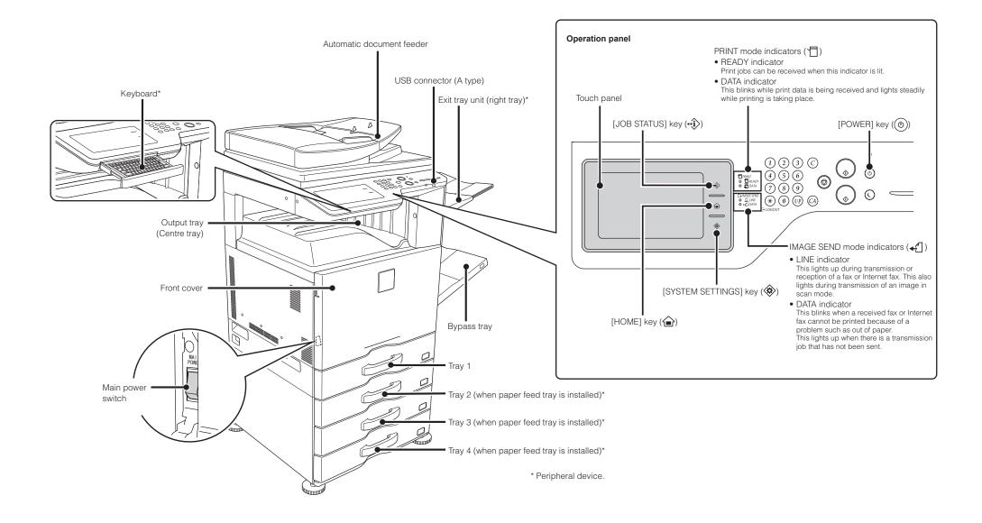
This machine has two power switches. The main power switch is at the bottom left after the front cover is opened. The other power switch is the [POWER] key ((()) on the operation panel.
