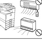
The paper will become damp and condensation may form inside the machine, causing misfeeds and dirty output. SPECIFICATIONS (page 10)
